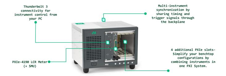
Make DC and impedance measurements in a seamless fashion with NI's PXIe-4190 - the world's first LCR Meter and SMU in a single instrument. This instrument provides femto-farad (10-15) class capacitance measurements and femto-amp current measurements in a single-slot PXI form factor. The new PXIe-4190 also removes the need for an additional switch to multiplex between the LCR Meter and SMU, allowing for a simplified test experience with higher throughput and lower capital cost.
